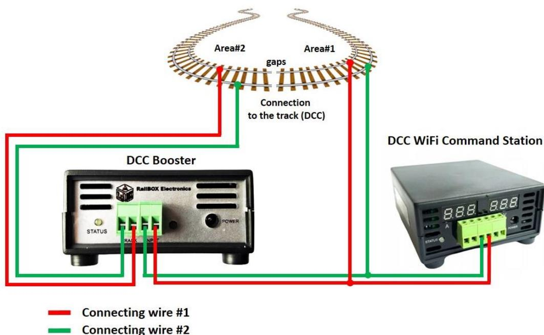
**Note:** DCC Booster can be used for controlling locomotives on the separate independent track area; this way each rail should be connected parallelly (wire from left pin output to left rail; right to the right) to the Booster and to the Command Station to avoid a short cut and/or any kind of damage of accessory decoders, during the moment when locomotive will be at both track areas at the same time when passing the gaps.
