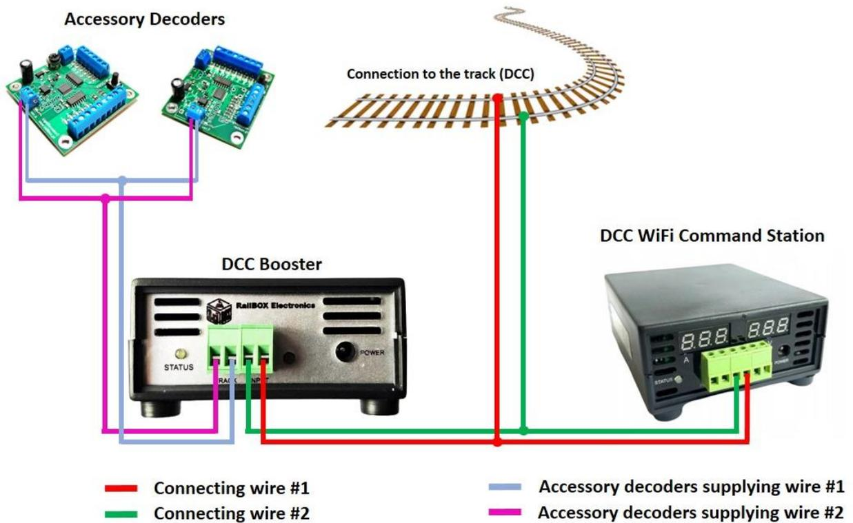
Note: DCC Booster as well can be used as supplying source for any of your accessory decoders.
